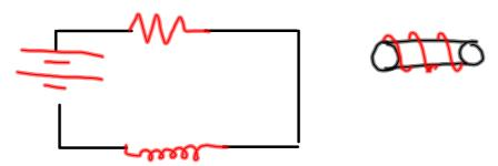
Time Constant: the time required for the current in the circuit to reach 63.2% of its final value E/R
