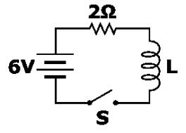
What is the current through inductor *L* long after the switch is closed?
