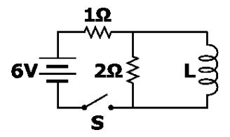
What is the current through the inductor L just after the switch is closed?
