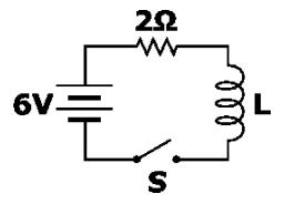
What is the voltage across inductor *L* just after the switch is closed?
