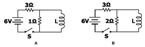
At t = 0, both switches are opened. Which resistor dissipates more total energy after the switches are opened?
