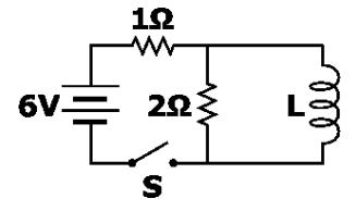
What is the current through inductor *L* long after the switch is closed?
