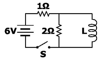
What is the voltage across inductor L just after the switch is closed?
