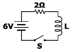
What is the current through the inductor L just after the switch is closed?
