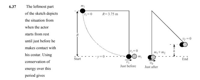
$$\left(KE + PE\right)_{1} = \left(KE + PE\right)_{i}$$
