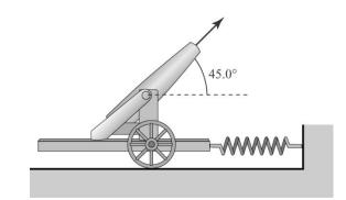
$$v_{\text{recoil}} = -\left(\frac{m_{\text{shell}}}{m_{\text{cannon}}}\right) v_{\text{shell}} \cos 45.0^{\circ}$$
