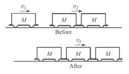
$$v_f = \frac{1}{3} \left( v_1 + 2v_2 \right)$$
