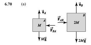
(b) From Newton's third law, the force  $\vec{\mathbf{F}}_{BA}$  exerted by *B* on *A* is at each instant equal in magnitude and opposite in direction to the force  $\vec{\mathbf{F}}_{AB}$  exerted by *A* on *B*.
