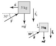
$$F = \frac{mg}{\sin 30^\circ - \mu_k \cos 30^\circ} = \frac{5.0 \text{ kg} \quad 9.80 \text{ m/s}^2}{\sin 30^\circ - 0.30 \cos 30^\circ} = 2.0 \times 10^2 \text{ N}$$
