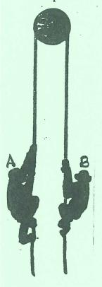
8. Refer to the drawing. Two unequal weights are suspended over a pulley. Which way will the system of weights move? Calculate the acceleration of each weight. What do you think the tension in the cable will be?
