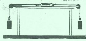
5. If a heavy object is suspended as shown, and the bottom string is pulled sharply, which string will break? Explain. What is the result if the bottom string is pulled with a slow, even motion? Explain.
